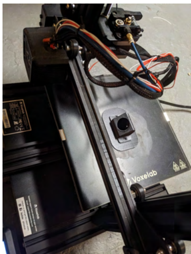
3D printing the motion sensor housing.
